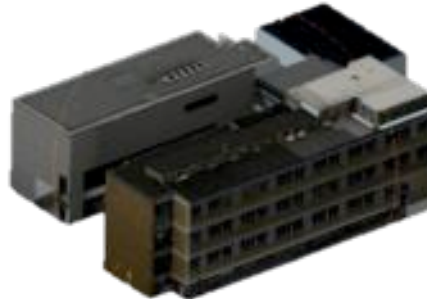
Figure 4: 3D image of a building complex obtained from stitching a large number of photographic images taken by a MAV
