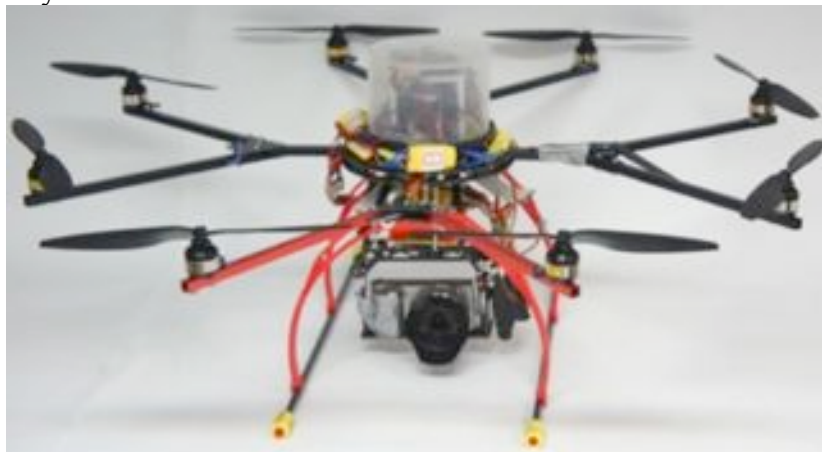
Figure 3: Example of an octo-copter equipped with a digital camera system
